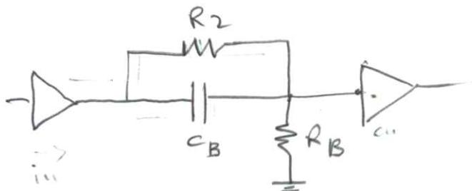
$$H_B = \frac{R_B}{R_B + R_2} \cdot \frac{1 + j\omega R_2 C_B}{1 + j\omega C_B R_B // R_2}$$
