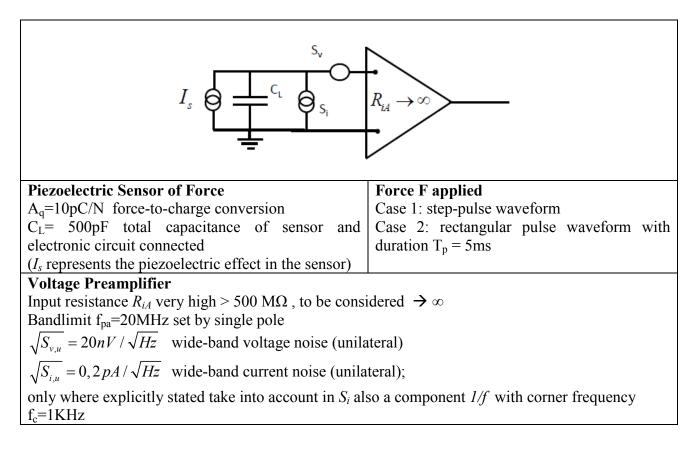
A piezoelectric force sensor connected to a voltage preamplifier with the characteristics above reported is employed for measuring the force applied to the sensor in the cases below specified. A suitable electrical filtering is applied to the sensor-amplifier output for improving the S/N.
