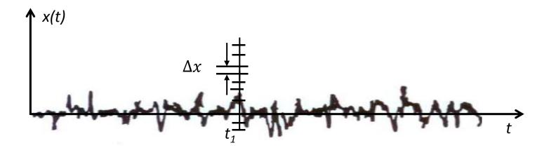
The amplitude  $x(t_1)$  of the noise waveform at time  $t_1$ is compared to a scale of discrete values  $x_k$  spaced by constant interval  $\Delta x$ and is classified at the nearest value  $x_k$  of the scale A high number N of noise waveform is sampled and measured of which  $\Delta N_k$  is the number of sample waveforms classified at  $x_k$  $\Delta f_k = \frac{\Delta N_k}{N}$  is called <u>statistical frequency</u> of the amplitude  $x_k$
