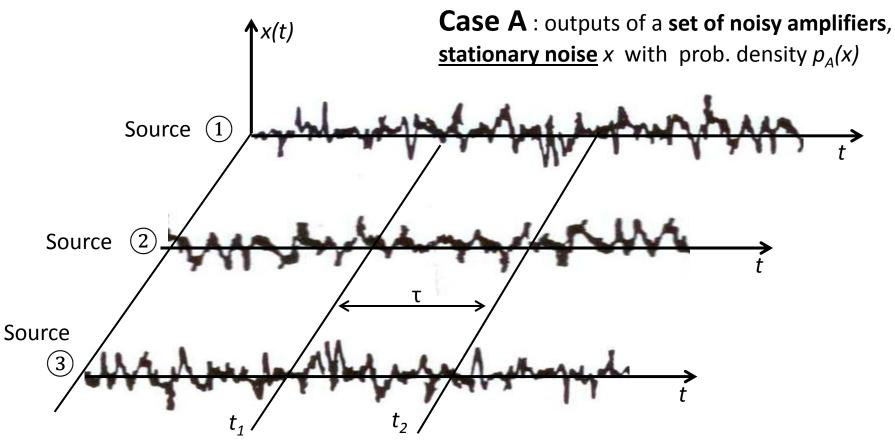
Values  $x(t_1)$  and  $x(t_2)$  measured on a sample waveform at different  $t_1$  and  $t_2$  are random values with equal probability density  $p_A(x)$  and they are
