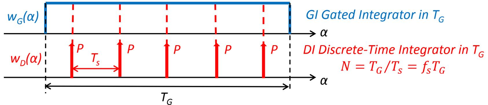
INPUT: DC signal  $s_x$  and wide-band noise  $S_b$  (bandwidth  $2f_n \gg f_s$ , correlation width  $2T_n \ll T_s$ ) with rms value  $\overline{n_x^2} = \sqrt{S_b 2f_n} = \sqrt{S_b/2T_n}$
