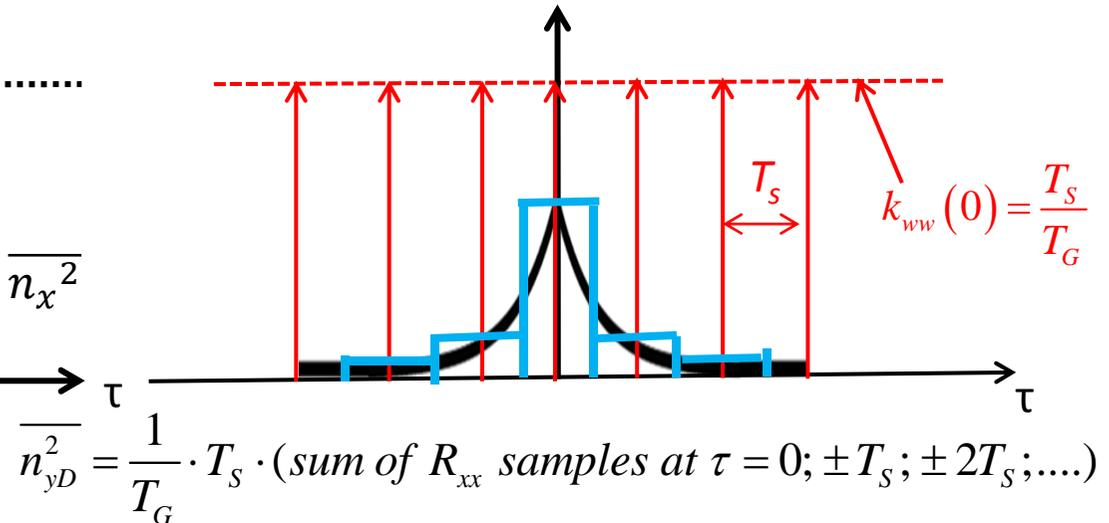
$$\overline{n_{yD}^2} = \frac{1}{T_G} \cdot (\text{area of the scaloid that approximates } R_{xx})$$
