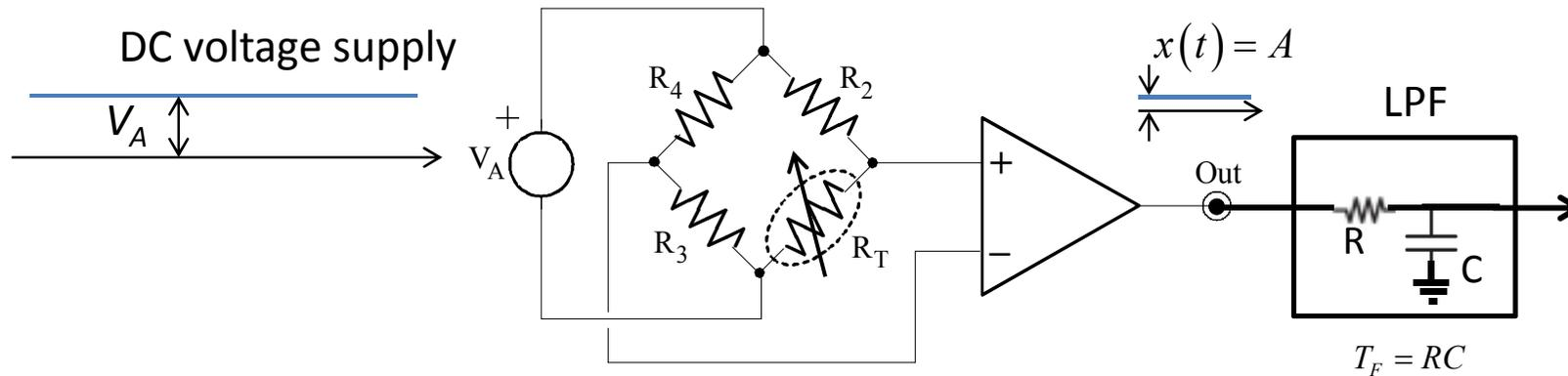
Let us consider the set-up of the key example (measurement with resistive sensor) now with DC supply voltage  $V_A$  equal to the amplitude of the previous AC supply. The signal now is a DC voltage equal to the amplitude  $A$  of the previous AC signal.
