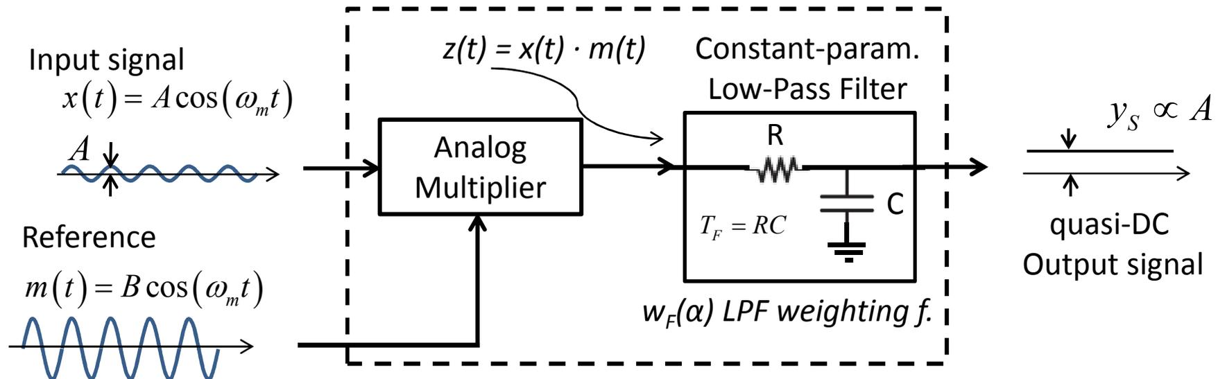
The **constant** parameter LPF performs a **running** average of  $z(t)$  over a few  $T_F$  that continuously updates the output
