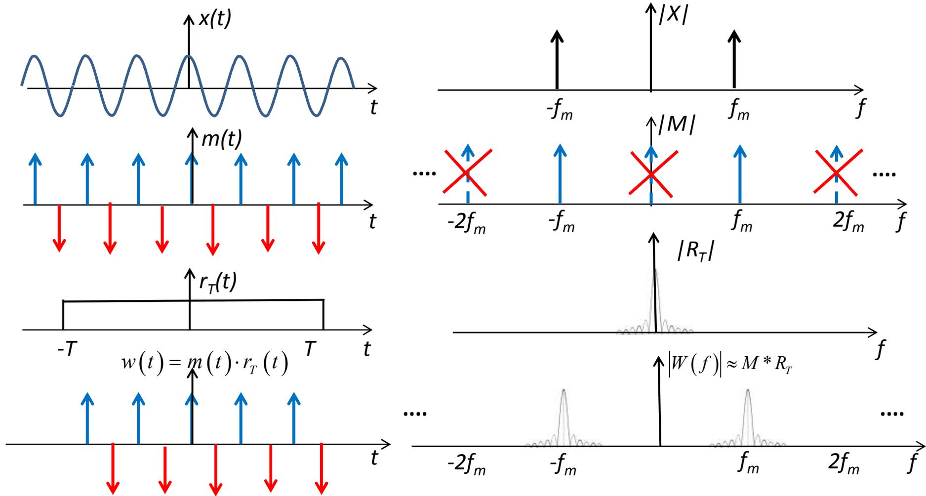
**FILTERING** : narrow bands at  $f_m$  and at **odd** multiples  $3f_m, 5f_m, \dots$
