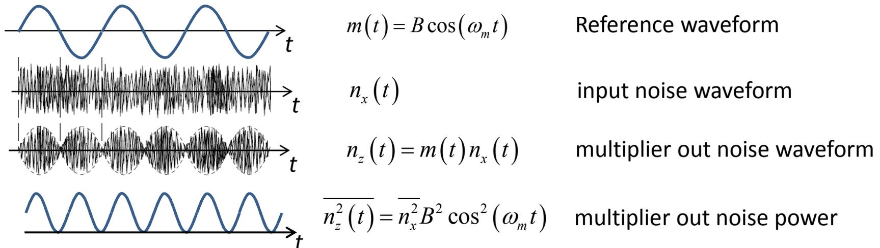
However, we will show that the LIA **output noise power** can be computed with an equivalent **stationary** noise, namely with the **average in time** of the cyclostationary noise
