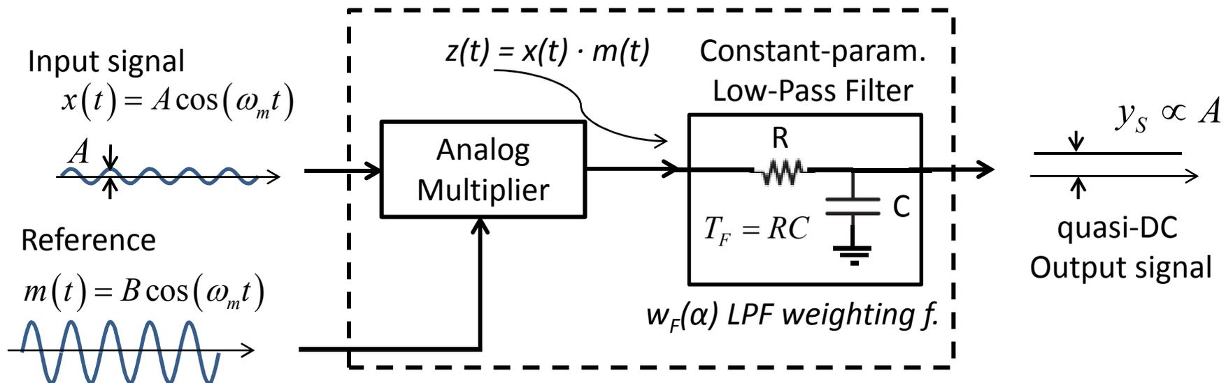
The **constant** parameter LPF performs a **running** average of the output  $z(t)$  of the demodulator. The output is continuously updated and tracks the slowly varying amplitude  $A(t)$ . This basic set-up is denoted Phase-Sensitive Detector (PSD) and is the core of the instrument currently called **Lock-in Amplifier**.
