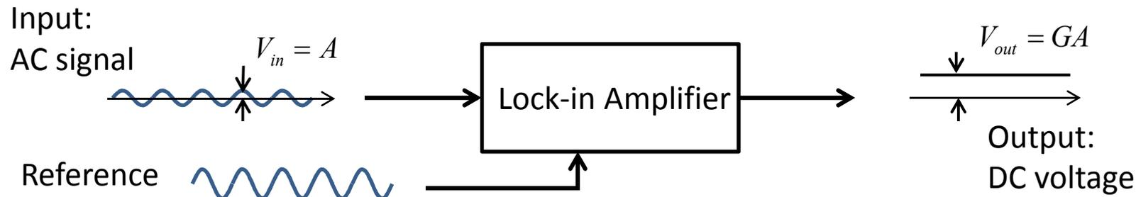
LIA Gain  $G = \frac{\text{output voltage}}{\text{input voltage}} = \frac{V_{out}}{V_{in}}$  however  $\begin{cases} V_{out} \text{ is a DC voltage} \\ V_{in} \text{ is the amplitude of an AC voltage} \end{cases}$
