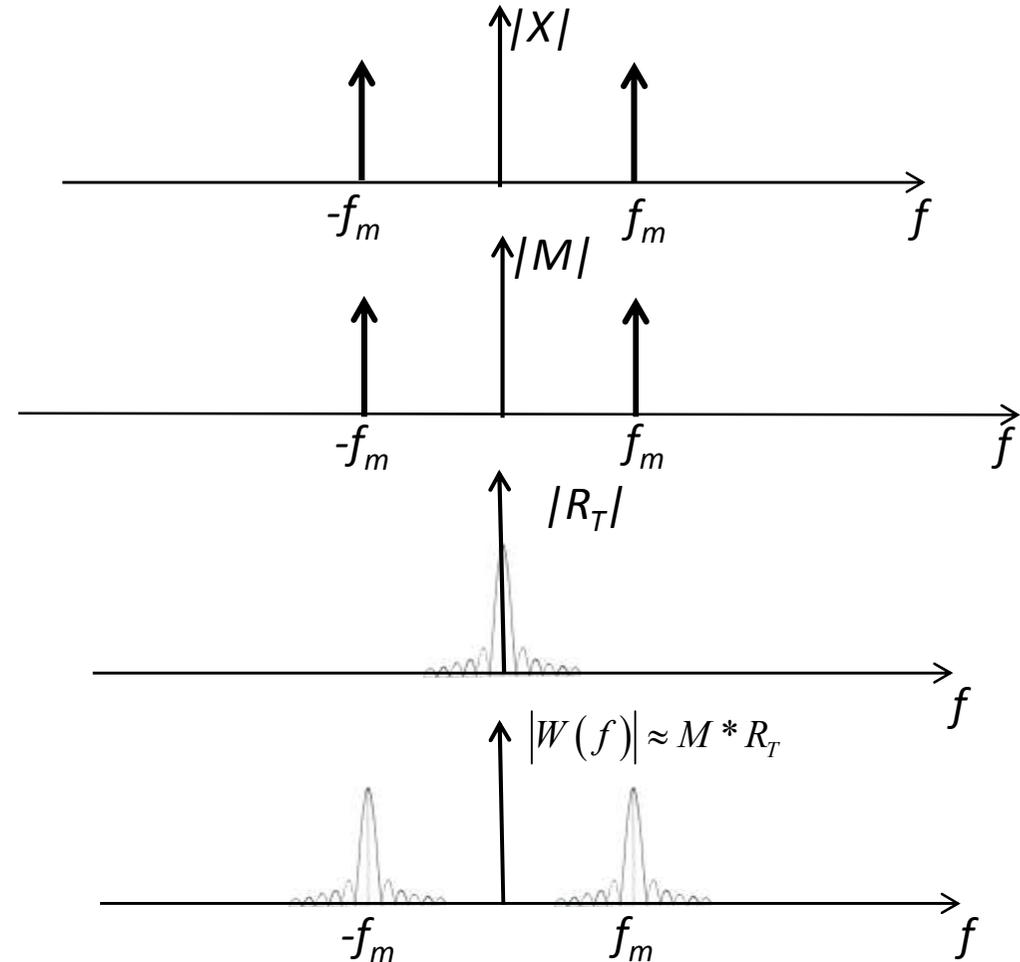
**TRULY EFFICIENT FILTERING : just one narrow band at  $f_m$**
