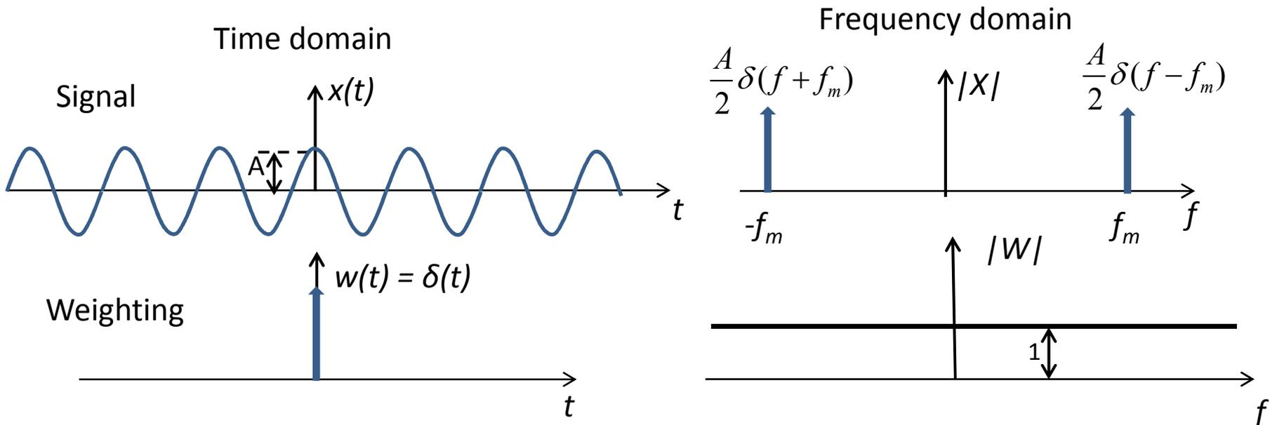
**NO FILTERING ACTION: output noise power = full input noise power**
