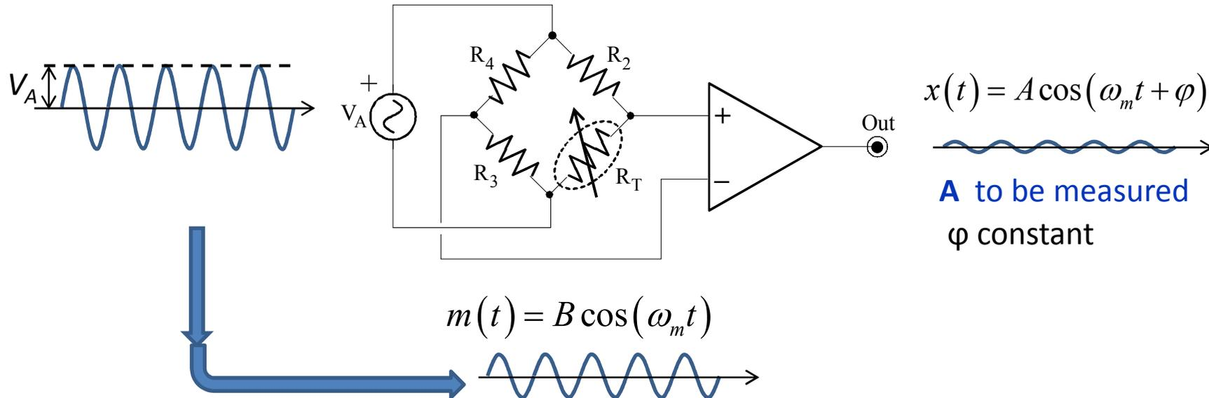
$R_T$  e.g. strain sensor, the resistance varies following a mechanical **strain**  $\vartheta$
