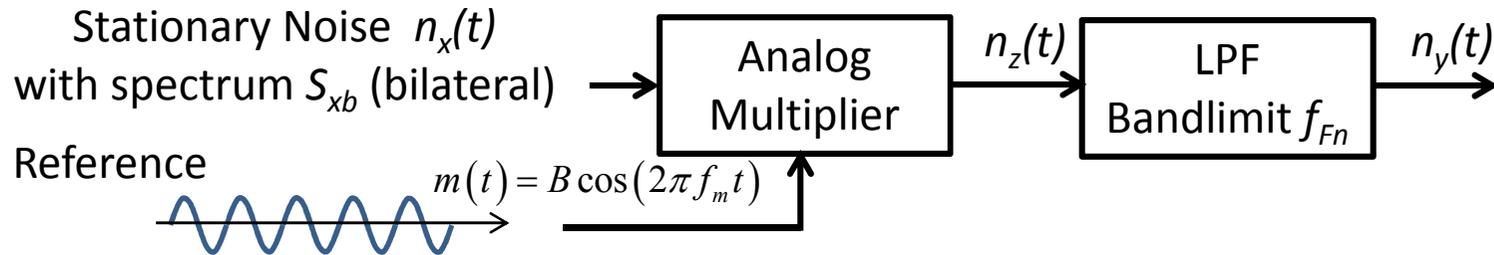
We might think that the **noise spectrum at the multiplier output** is simply the superposition of two replicas of the **input spectrum shifted up and down by  $f_m$** , but this is not exactly the case. The input noise  $n_x(t)$  is stationary, whereas the multiplier output noise  $n_z(t)$  is **not stationary**, it has cyclically varying intensity so that it is denoted «**cyclostationary**» noise
