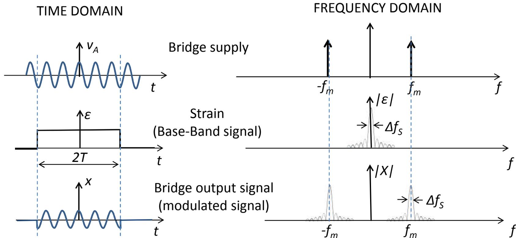
1. The Base-band signal is not constant, it is slowly variable, hence the modulated signal has a **finite bandwidth  $\Delta f_s$  around  $f_m$**
