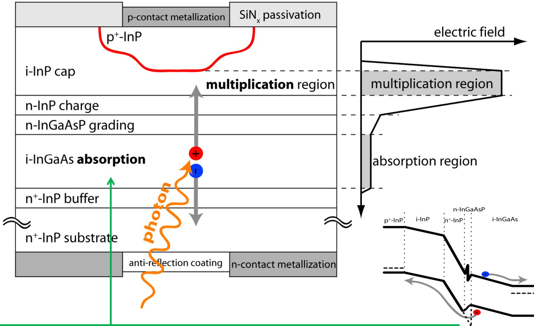
In<sub>0.53</sub>Ga<sub>0.47</sub>As absorption layer → E<sub>g</sub> ~ 0.75 eV → Cut-off 1.7 μm
