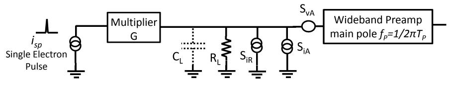
The circuit noise components in voltage referred to the amplifier input are  $\sqrt{S_{vA}} \approx 4 \, nV / \sqrt{Hz}$ ;  $R_L \sqrt{S_{iA}} = 0, 2 \, nV / \sqrt{Hz}$ ;  $\sqrt{S_{vR}} = \sqrt{4kTR_L} \approx 0,9 \, nV / \sqrt{Hz}$
